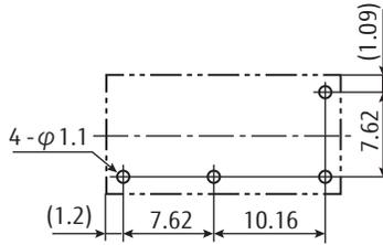
Tolerance of PC board mounting hole layout:  $\pm 0.1$  unless otherwise specified.
