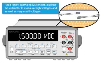
Figure 2. Reed Relay switch contacts are open.
