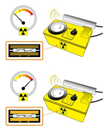
Figure 2. Reed Relays switch low signals in electrometers.
