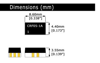
Figure 1. CRF physical layout
