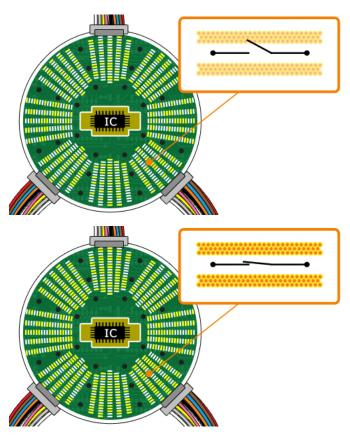
Figure 2. This is a typical performance board which is usually loaded with relays circling the center, which is where the IC is tested.
