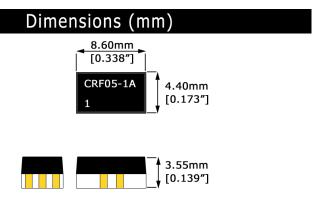
Figure 1. CRF physical layout
