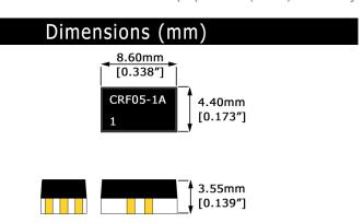
Figure 1. CRR/CRF physical layout
